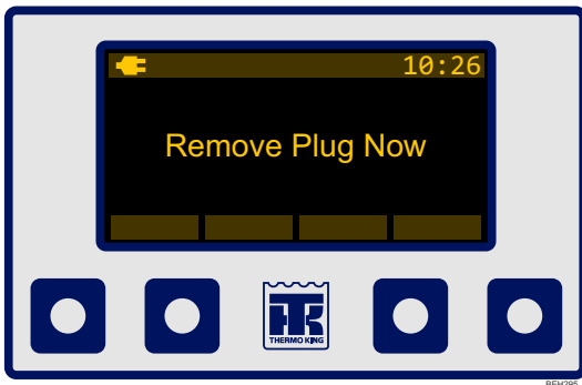
Figure 14. Safe removal of shore power plug: Message on HMI
