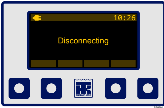
Figure 13. Disconnecting shore power: Message on HMI
