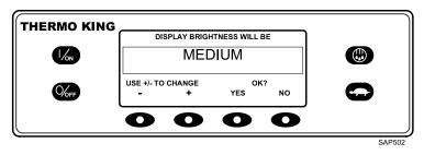
The display will briefly show ADJUSTING BRIGHTNESS - PLEASE WAIT. The display brightness is changed to the new setting. To return to the Main Menu press the EXIT soft key. To return to the Standard Display press the EXIT soft key again.
