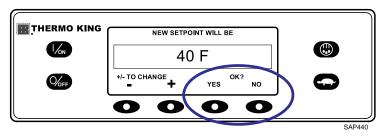
After the YES soft key has been pressed, the display briefly shows PROGRAMMING NEW SETPOINT - PLEASE WAIT. The display then confirms the new setpoint for several seconds.
