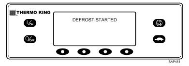
The display then shows the Defrost display. The bar indicator shows approximately how much time remains to complete the defrost cycle. The bar indicator (Figure 42, p. 45) shows that the defrost cycle is about 25% complete.
