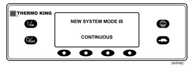
The display then returns to the Mode Menu. In the example shown (Figure 85, p. 74), the unit is currently running in Continuous Mode. Pressing the
