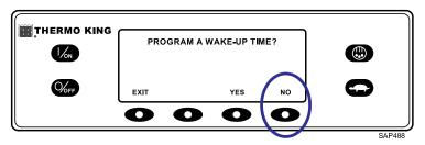
The display will show SLEEP and the unit will start and stop as required to keep the engine warm and/or the battery charged. To exit Sleep Mode, press the EXIT key or turn the unit off and back on. The unit will resume normal operation and control to setpoint.
