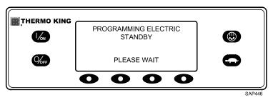
Electric Mode operation will briefly be confirmed. If unit operation is required, the electric motor will start as shown in Starting The Electric Motor.
