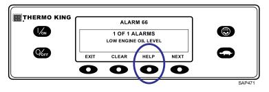
A help message will appear. For the alarm shown (Figure 68, p. 61), the message "CHECK OIL LEVEL. IF UNIT IS SHUT DOWN, REPAIR IMMEDIATELY. OTHERWISE, REPORT ALARM AT END OF THE DAY" will be shown on the display. Check the oil level and add oil as required, clear the alarm and restart the engine.
