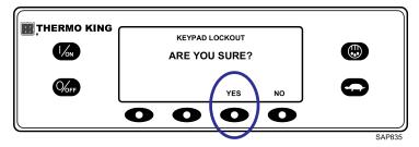
After the YES soft key has been pressed, the display will briefly show KEYPAD LOCKED. The display confirms the setting for two seconds and then returns to the Locked Standard Display.
