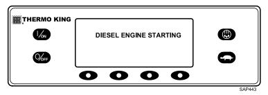
After the engine is started, the display returns to the Standard Display of temperature and setpoint.
