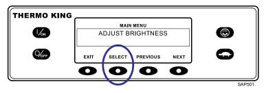
The Display Brightness menu will appear as shown (Figure 116, p. 89). Press the + or - keys to select the desired display brightness. When the desired brightness is shown, press the YES key to confirm the choice.
