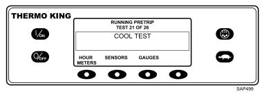
When all tests are complete, the results are reported as PASS, CHECK, or FAIL. If the results are CHECK or FAIL, the accompanying alarm codes will direct the technician to the cause of the problem. If the Pretrip Test results are CHECK or FAIL, the problem should be diagnosed and corrected before the unit is released for service.
