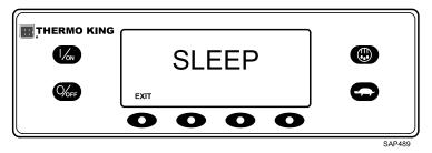
The unit will restart at the programmed time (in this example 4:30 am) and perform a Pretrip Test (if selected). After the Pretrip Test is complete, the test results will be displayed and the unit will resume normal operation and control to setpoint.
