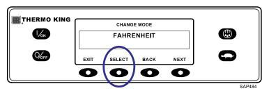
The Temperature Display screen will appear. Use the + and - soft keys to chose either FAHREHEIT or CELSIUS. When the desired temperature units are shown, press the YES soft key to select.
