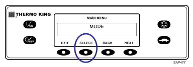
The first mode change screen will appear. To choose that function, press the SELECT key. To Scroll through the Mode Menu, press the NEXT key.
