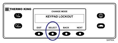
The Keypad Lockout Confirmation screen will appear. To enter Keypad Lockout Mode press the YES soft key to confirm the choice.
