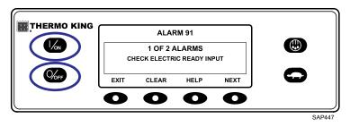
Turn the unit off and back on using the OFF and ON Keys. This will clear Alarm Code 91 Check Electric Ready Input and Alarm Code 84 Restart Null.
