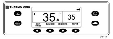
The CYCLE-SENTRY lcon in the upper right corner of the display shows that the unit is operating in CYCLE-SENTRY Mode. If the CYCLE-SENTRY lcon is not present, the unit is operating in Continuous Mode.
