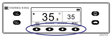
To exit Keypad Lockout Mode press and hold any of the soft keys for five seconds. Keypad Lockout Mode will be turned off and the Standard Display will appear.
