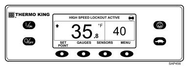
Pressing the High Speed Lockout key again will turn the feature off.
