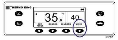
The Language Menu or Alarm Menu will appear. Press the NEXT key as required to display the Hourmeter Menu. When the Hourmeter Menu is shown, press the SELECT key. The Hourmeter Display will appear.
