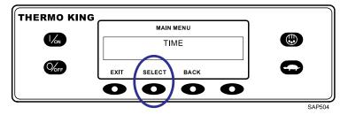
The current time and date will appear. To return to the Main Menu press the EXIT soft key. To return to the Standard Display press the EXIT soft key again.
