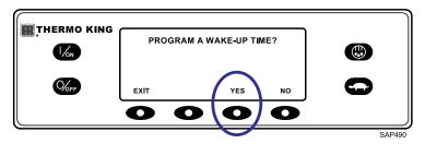
The display will prompt the operator for the DAY the unit is to restart in normal operation. In the example shown (Figure 102, p. 81), Monday has been chosen. Press the YES key to confirm the DAY.
