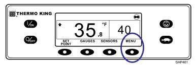
The Language Menu or Alarm Menu will appear. Press the NEXT key as required to display the Data Logger Menu. When the Data Logger Menu is shown, press the SELECT key.
