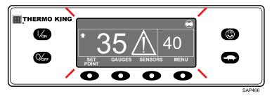
Shutdown Alarms will force the unit into shutdown to prevent potential damage to the unit or load. The unit will remain in shutdown until the Shutdown Alarm is manually cleared. Exceptions are some engine and electric Shutdown Alarms that become Log Alarms when switched to the alternate operating mode (diesel to electric or electric to diesel).
