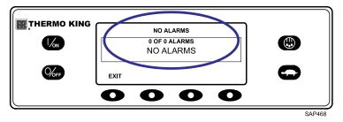
If alarms are present, the quantity of alarms (if more than one) and the most recent alarm code number will be shown. In the example shown (Figure 66, p. 60), there are two alarms present. The most recent is Alarm Code 6. It indicates a problem with the coolant temperature sensor.
