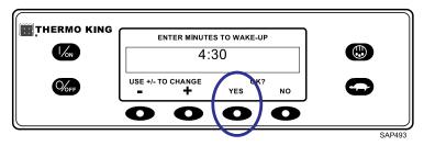
The display will now prompt for a Pretrip Test on Wake-up. Press the YES key to perform a Pretrip Test on Wake-up. If the No key is pressed, the unit will resume normal operation on Wake-up.
