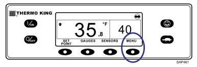
The Language Menu or Alarm Menu will appear. Press the NEXT key as required to display the Adjust Brightness Menu. When the Adjust Brightness Menu is shown, press the SELECT key.
