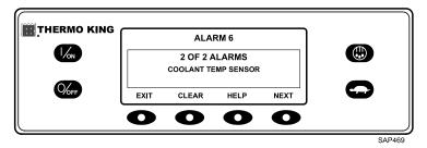
After the alarm situation is resolved, press the CLEAR key to clear the alarm. For additional information regarding the alarm shown on the display, press the HELP key. To display the next alarm, press the NEXT key.
