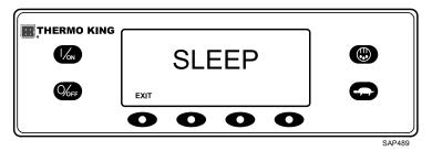
To enter a Wake-up Time, verify the unit clock is set properly. Press the YES key at the Sleep Mode Menu.
