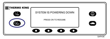
The display briefly shows OFF and then goes blank. To start the unit again, press the ON key.
