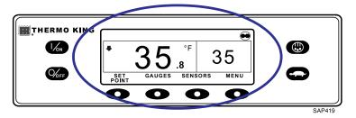
The Standard Display of box temperature and setpoint is shown (Figure 10, p. 29). The CYCLE-SENTRY Icon in the upper right of the display shows the unit is running in CYCLE-SENTRY (Start-Stop) Mode. The unit has a setpoint of 35°F, and an actual box temperature of 35.8°F. The down-pointing arrow at the left side of the display shows the unit is cooling.
