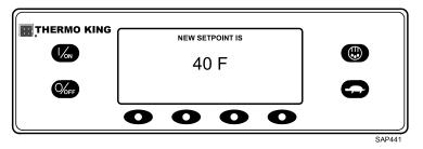
If the NO soft key is pressed, the display will briefly show SETPOINT NOT CHANGED and return to the Standard Display. The Standard Display will show the old setpoint. The display then returns to the Standard Display showing the new setpoint. The arrow now points up to indicate that the unit is heating (Figure 30, p. 39).
