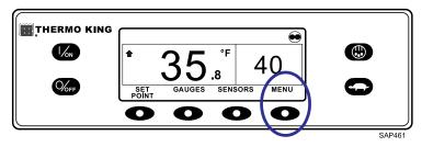
The Language Menu or Alarm Menu will appear. Press the NEXT key as required to display the Mode Menu. When the Mode Menu is shown press the SELECT key.
