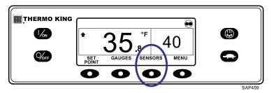
The first sensor display will appear. Press the NEXT and BACK keys to scroll through the sensors. The Discharge Air Temperature sensor is shown (Figure 50, p. 49). Press the LOCK key to lock the current sensor on the display.
