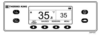
Pressing the OFF key stops unit operation. The unit shuts down immediately and the display briefly shows the power down message.
