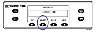
Press the NEXT or PREVIOUS key to scroll through the enabled hourmeters.
