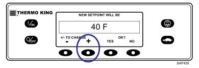
The YES and NO soft keys confirm the setpoint change. When the desired setpoint has been selected using the + and/or - keys, press the YES soft key to confirm and load the new setpoint. If the setpoint is changed using the + or - keys, the change must be confirmed or rejected by pressing the YES or NO soft key within 10 seconds of changing the setpoint.
