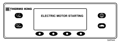
After the motor is running, the display returns to the Standard Display of temperature and setpoint.
