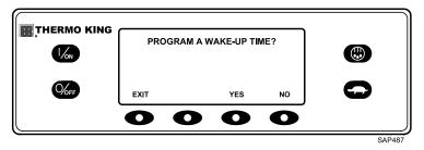
The operator can now choose a Sleep Mode Wake-up Time or simply enter Sleep Mode immediately. If NO is pressed, the unit will immediately enter Sleep Mode.
