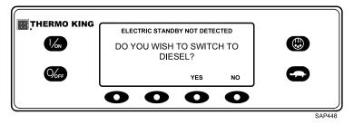
If YES is selected, the display will briefly show the programming screen (Figure 39, p. 43). Diesel Mode operation will briefly be confirmed.
