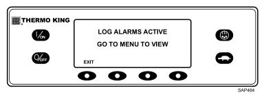
**Note:** If required, an engine start may occur while the Log Alarm Notice is shown (Figure 60, p. 55). This is normal operation.
