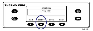
If the unit is not running, a Full Pretrip Test will be initiated. If the unit is running in either diesel or electric mode, a Running Pretrip will be performed.
