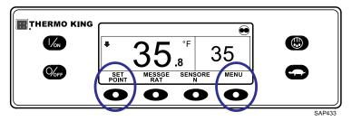
The Language menu will appear in the current language as shown (Figure 20, p. 34). Press the + or - keys to select the desired language. When the desired language is shown, press the YES key to confirm the choice. All languages in the installed software can be selected using this method.
