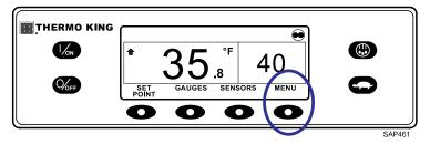
The first Main Menu choice will appear. Press the NEXT and BACK keys to scroll through the menu choices. When the desired selection is shown on the display, press the SELECT key to access it. The Pretrip submenu is shown (Figure 52, p. 51). To return to the Standard Display press the EXIT key.
