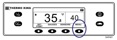
The Language Menu or Alarm Menu will appear. Press the NEXT key as required to display the Time Menu. When the Time Menu is shown, press the SELECT key.
