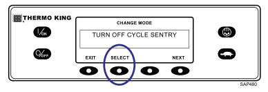
The display will confirm the change as shown (Figure 83, p. 73).
