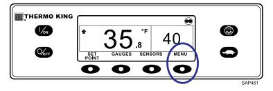
The Language Menu or Alarm Menu will appear. Press the NEXT key as required to display the Mode Menu. When the Mode Menu is shown press the SELECT key.
