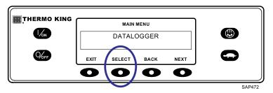
The first feature that appears is the Start of Trip. To send a Start of Trip to the ServiceWatch Data Logger and DAS Data Logger (if equipped), press the SELECT key to select the feature, and press it again to send the Start of Trip. The display will briefly show START OF TRIP COMPLETE to confirm that a Start of Trip marker was set in the data logger(s).
