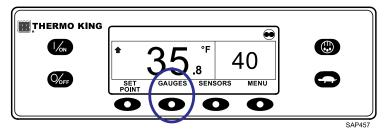
The first gauge display will appear. Press the NEXT and BACK keys to scroll through the gauges. The Battery Voltage Gauge is shown (Figure 48, p. 47). Press the LOCK key to lock the selected gauge on the display.
