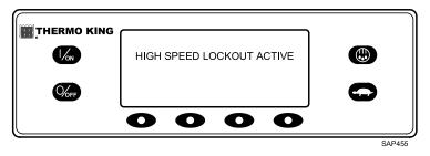
The display will then return to the Standard Display. If High Speed Lockout is turned on, the message HIGH SPEED LOCKOUT ACTIVE will be shown at the top of the display.
