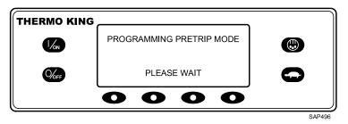
If all alarms were not cleared, a prompt appears as shown (Figure 110, p. 86). Exit the Pretrip Test, clear all alarms, and restart the Pretrip Test.
