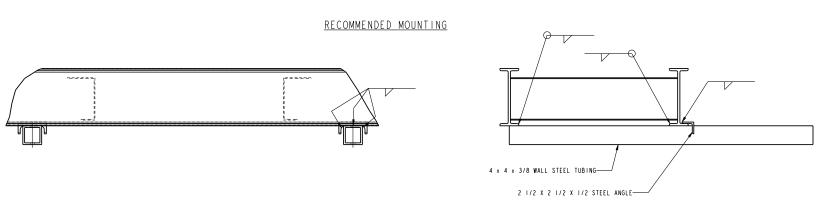
ATTACH GENSET WITH 5/8-II, GRADE 5 HARDWARE TORQUE TO 150 FT-LBS.
