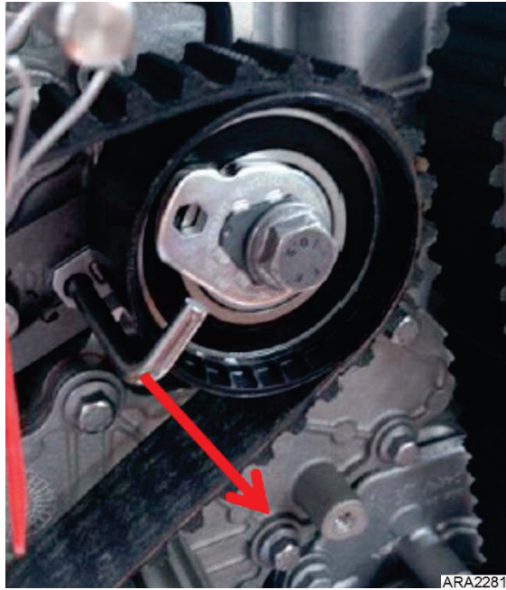
Figure 58. Remove Shipping Key from Belt Tensioner
