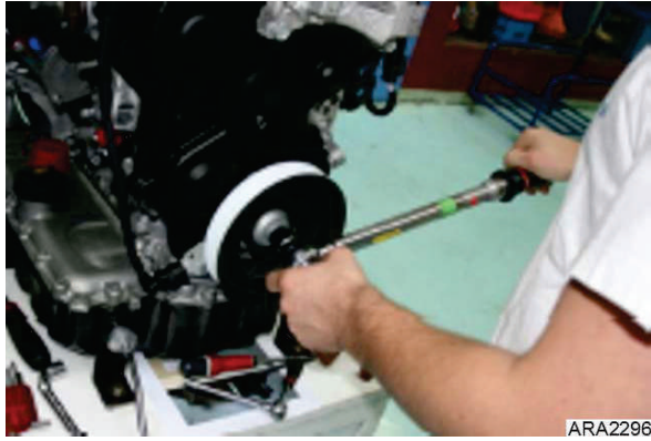
Figure 73. Torque to 25.8 ft-lb (35 N•m)
