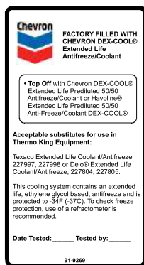
Figure 3. ELC Nameplate Located Near Expansion Tank
