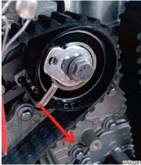
Figure 58. Remove Shipping Key from Belt Tensioner
