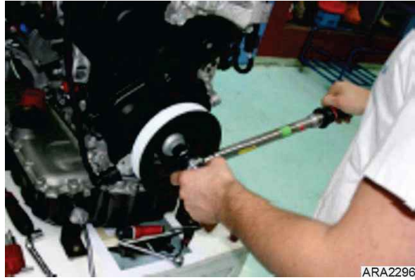
Figure 73. Torque to 25.8 ft-lb (35 N•m)
