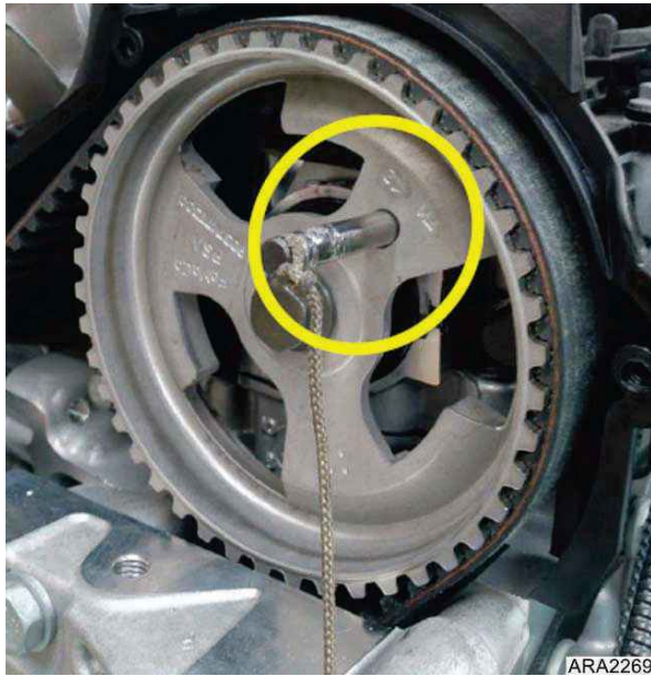
Figure 44. Place Peg in Camshaft and Cylinder Head
