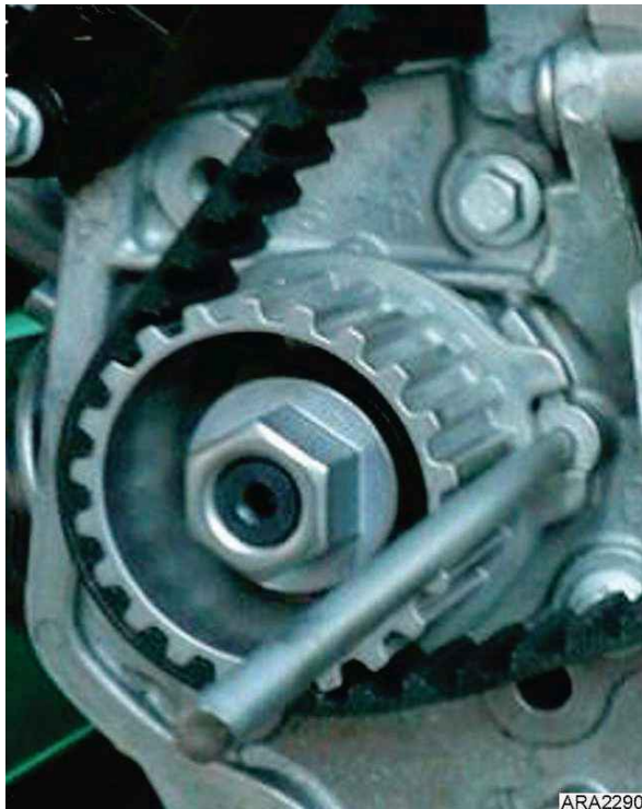
Figure 67. Install Pin P/N 204-2977 at Injection Pump Pulley
