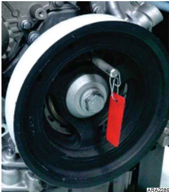
Figure 66. Peg Crankshaft with Tool P/N 204-2977
