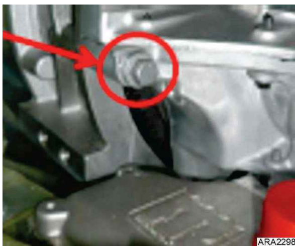
Figure 76. Torque to 40.6 ft-lb (55 N•m)
