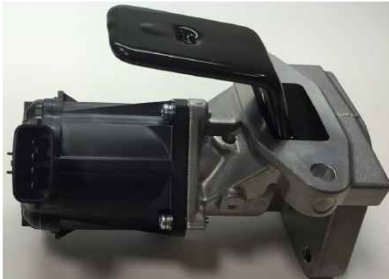
Mechanical EGR Tool shown properly positioned into the side opening of EGR valve.
