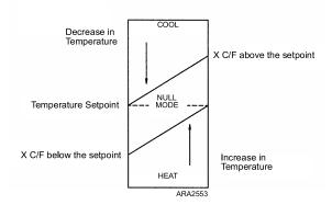
Factory setting for X is  $3^{\circ}$ C ( $5^{\circ}$ F). During unit installation, this value can be adjusted by between 1 and  $5^{\circ}$ C (2 and  $9^{\circ}$ F) in increments of  $1^{\circ}$ C/F.
