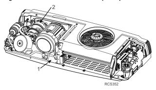
Figure 13. Engine Driven Compressor Serial Number Location
