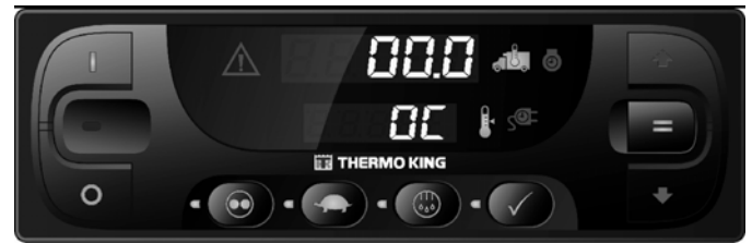
Figura 6: Painel de controlo HMI Standard
