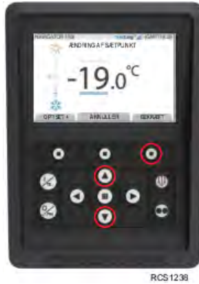
Figur 29. Displayet Termostatindstilling vist
