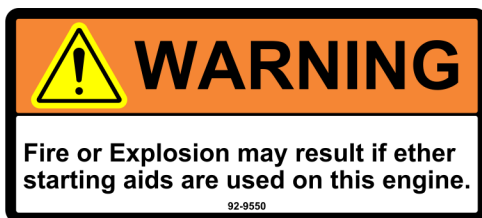
Figure 5. Do Not Use Ether Starting Aids (Near Engine)
