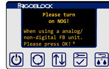
thermostat can be switched on and off at the second remote control unit. It is also possible to manually start defrost mode of the refrigeration device
