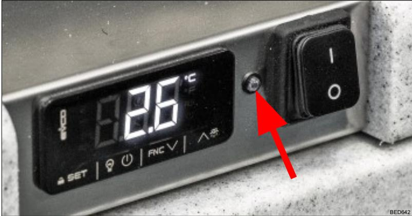
Each flash will last 1/4 second. After the actual number of flashes there will be a delay with no flashes, so that the sequence for each error recording is repeated every 4 seconds.
