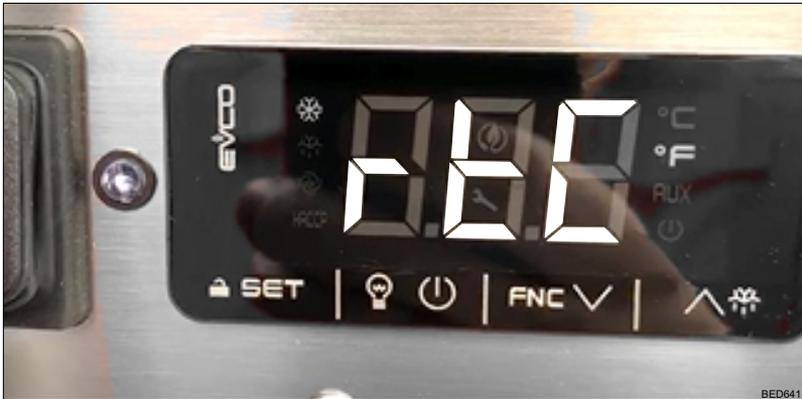
The real time clock is a function not included in the EV3294 installed in the ColdCube™ Connect, it is included in the EVlink Bluetooth module 510012/00.
